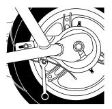
**2** With a 10mm wrench, loosen the brake cable anchor and disconnect the brake cable.
